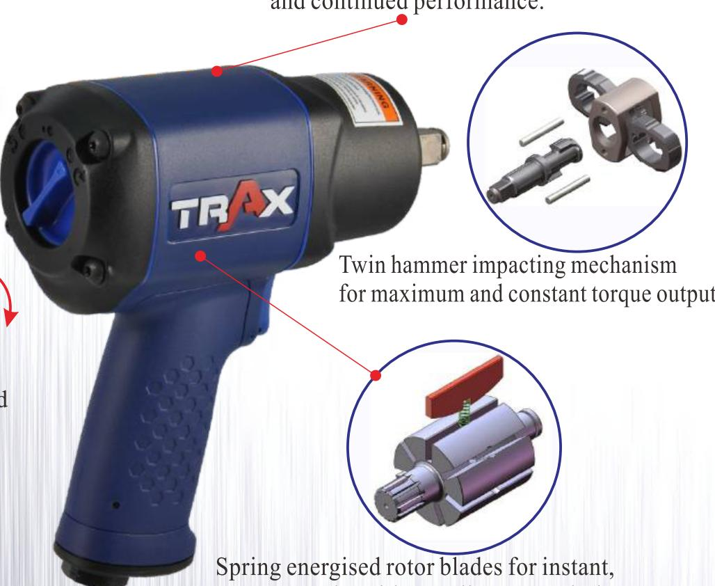
Spring energised rotor blades for instant, constant and positive sealing to maximise power.
